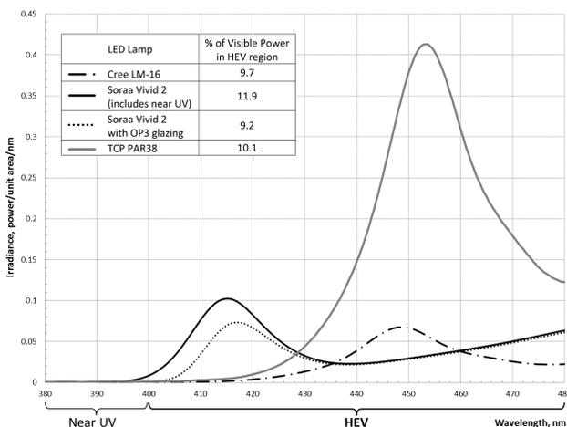
Figure 6: Spectra of LEDs in the HEV region
