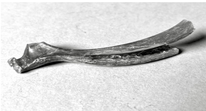
Cleaving and distortion of plastic in opposing directions © Academy Museum Foundation
